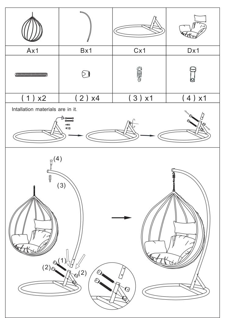
Note: All the installation materials are put in the tube of base.
